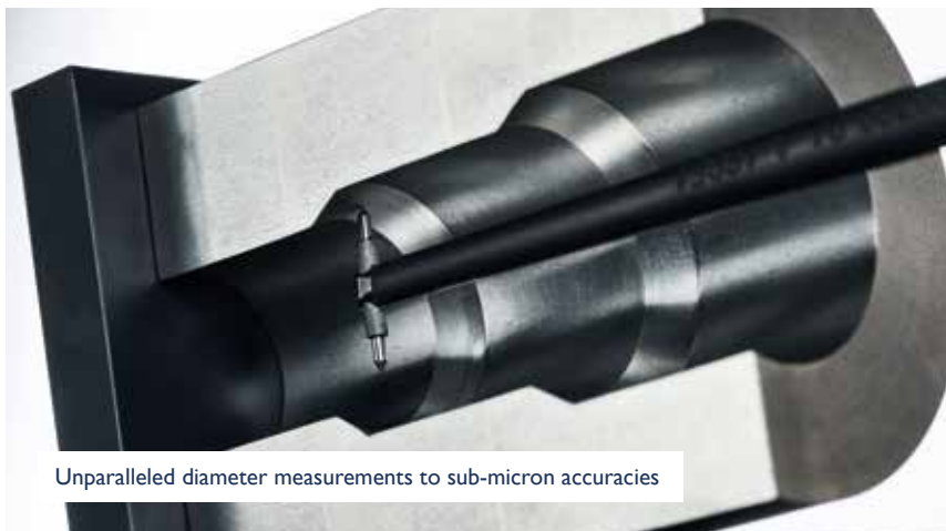
Internal raceway diameter, form and roughness
