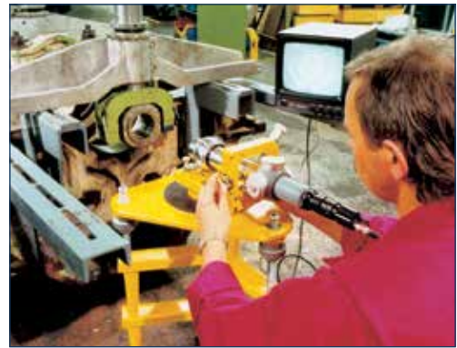
Diesel engine alignment (shown here using camera system 137-2161-01)
